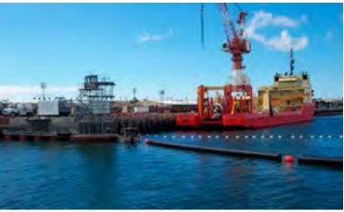
A simple, lower cost demarcation barrier of 0.5 or 1 m diameter is available where port vessel movement control is required such as around piers and pipeline jetties.
