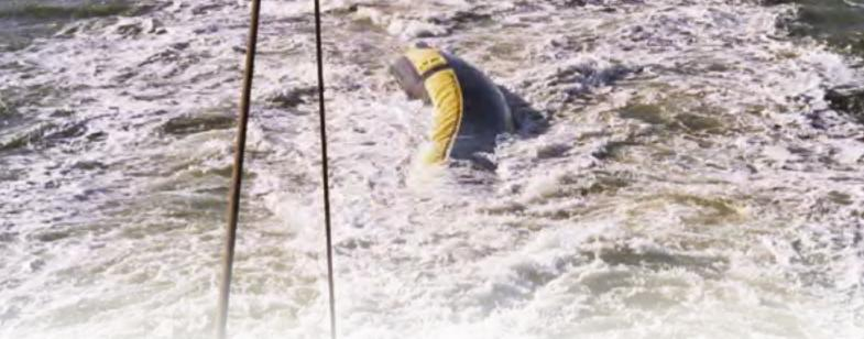
**Strong and reliable under harsh conditions** - The Dracone barge is constructed from synthetic rubber-coated nylon fabric, making it highly resistant to all weather conditions, abrasion, sunlight, oil and sea water.
