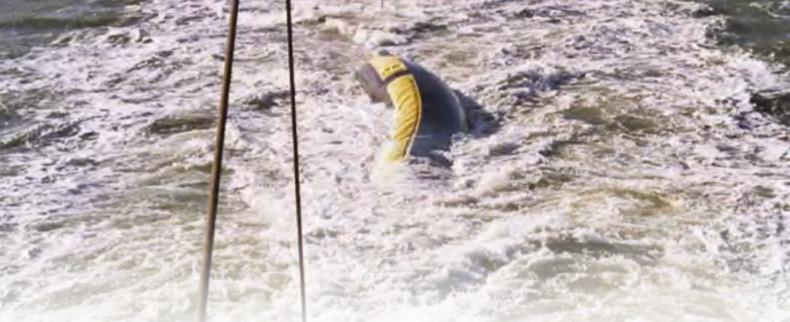
**Strong and reliable under harsh conditions** - The Dracone barge is constructed from synthetic rubber-coated nylon fabric, making it highly resistant to all weather conditions, abrasion, sunlight, oil and sea water.
