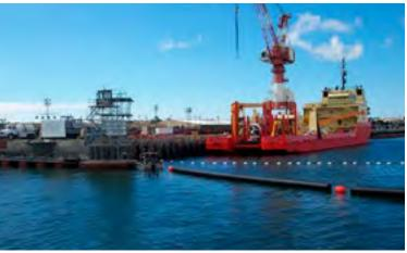
A simple, lower cost demarcation barrier of 0.5 or 1 m diameter is available where port vessel movement control is required such as around piers and pipeline jetties.
